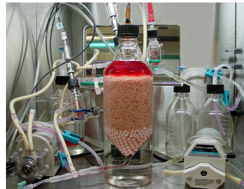
Fig. A packed-bed type bioartificial liver system.
